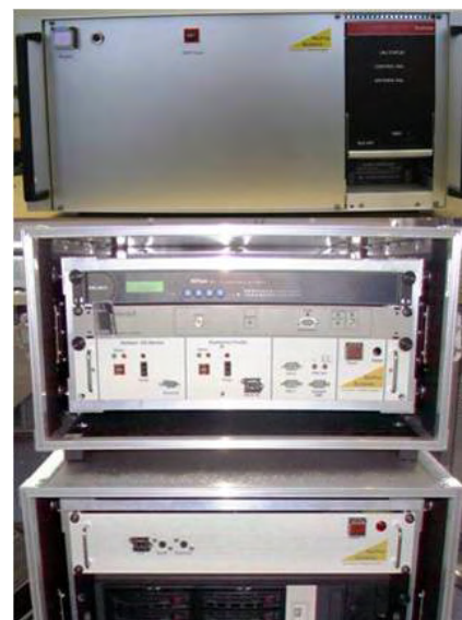
The independent GBAS monitoring system UGM consists of three components: a server unit (below), a GNSS unit (middle), and an MMR unit (above).
